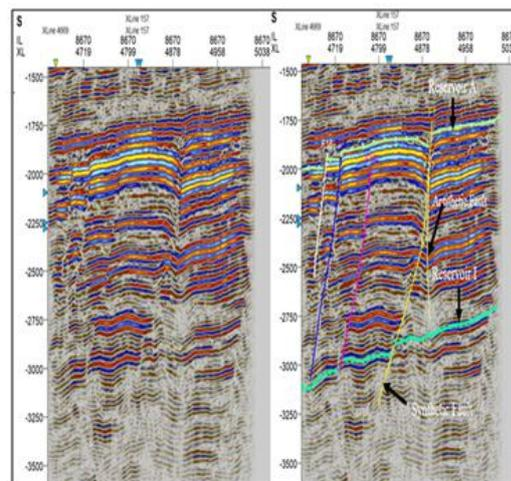
Figure 5: Faults and horizon interpreted along seismic inline section (a) Original seismic, (b) faults and horizons interpreted
